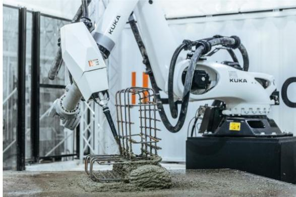
Industrial robots that automate the manufacturing process of concrete precast elements in its entirety – from concrete batching to post-processing (Image: Aeditive)
